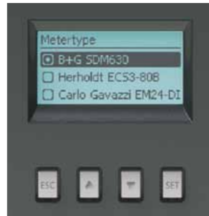
Quick and easy installation: pre-programmed energy meters are easily selected using the inverter's display.
